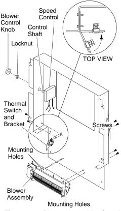
Figure 17 - Blower Assembly, Speed Control, and Thermal Switch Locations
